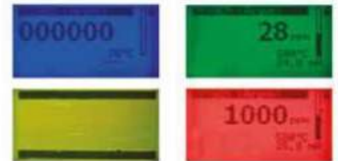
Colour changing display for quick reference to monitor status
