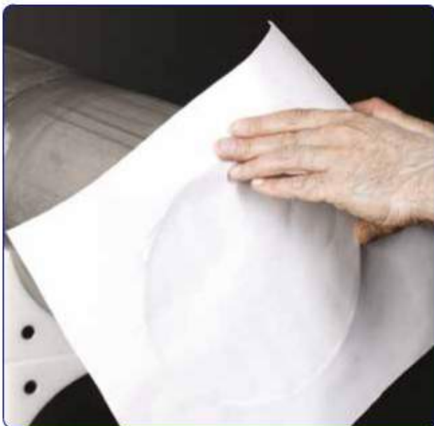
Impress the pipe i/d on the paper
