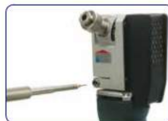
Precise adjustment of the stick-out
