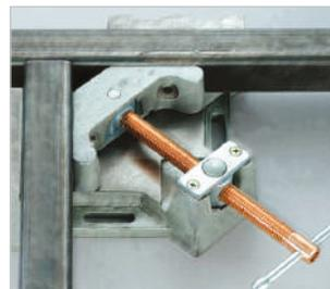
▶ Open design makes it possible to clamp T joints
