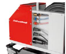
All connections on the intermediate hose pack are easily accessible and pluggable without tools
