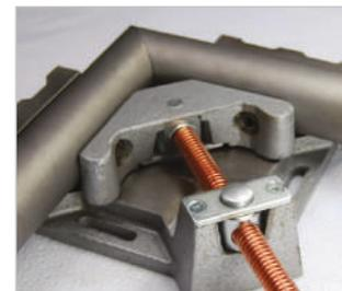
▶ Also suitable for clamping round material
