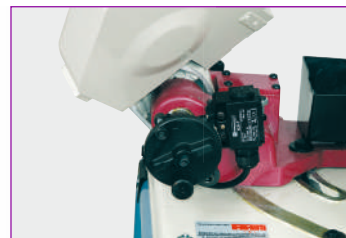
Automatic limit switch cut-off › Switches the saw band off at the bottom stop
