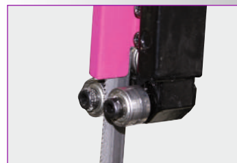
Saw band guide › Ball-bearing borne 3-point guide
