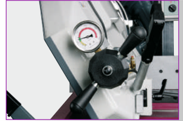
Pressure gauge › Easy and accurate adjustment of the saw band tension
