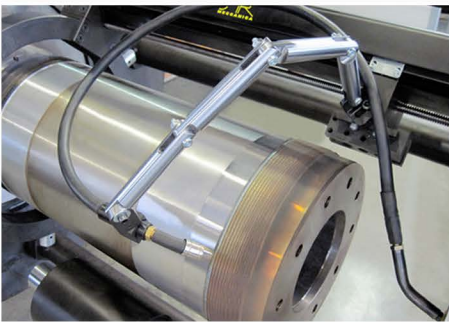
External Overlay welding
