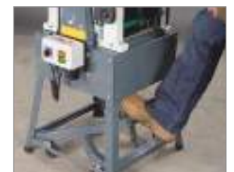
The factory standard chassis with two steering rollers ensures ease of transport. To move the machine, simply step on the chassis bar, which moves the rollers down. The chassis is then returned to its original position by a spring-loaded bar.
