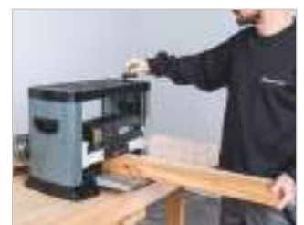
Height adjustment via crank and scale
