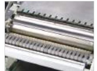
Automatic, uniform feed with anti-kickback device. The geared infed roller guarantees a constant wood feed speed.
