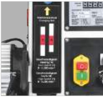
Variable speed control from 0 - 1 200 rpm (L) and 0 - 3 200 rpm (H) in two
