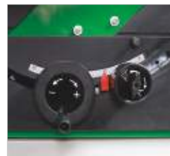
Precise, easy-action height and angle adjustment of the sawing unit via easily operable handwheels
