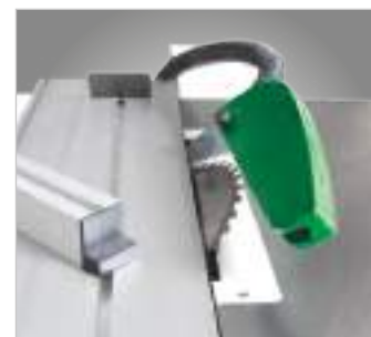
The saw blade pivots through 45°.
