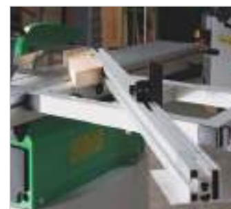
Pivoting telescope stop on sliding carriage; extendable to 2 280 mm, and foldable
