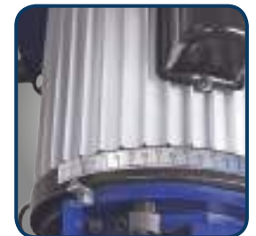
Sanding arm of belt sanding machine pivots from 0 - 90° thanks to clamping screw and scale
