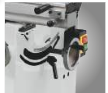
Saw blade pivots from 0° to 45°, easily adjustable via gear rack mechanism with rotary knob and scale
