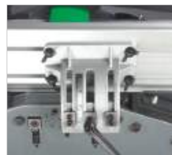
The aluminium jointing stop pivots continuously through 45°. The preset angle can be read off on a scale. (Fig. shows ADH 250)
