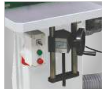
Height-adjustable sanding table utilises the entire width of the sanding belt
