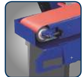
Easy belt run adjustment via knurled screw
