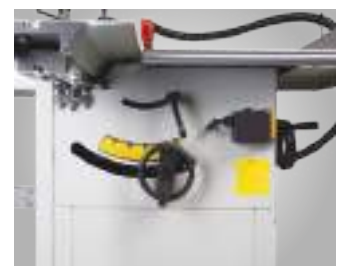
Saw blade pivots from 0° to 45°, easily adjustable via gear rack mechanism with rotary knob and scale
