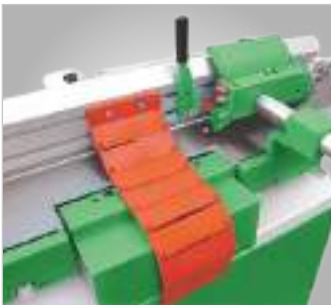
Planing shaft cover for safe working
