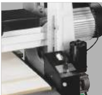
Height adjustment of the sanding unit can be read off on a scale
