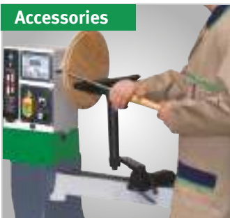
The headstock can be pivoted for turning workpieces in cross grain operations that are larger than the inside dimension of the lathe. The optional bed extension in combination with the convertible manual tool support ensure maximum flexibility.
