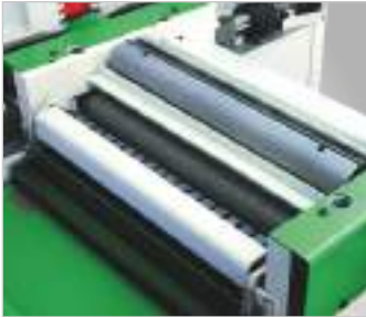
Precision-borne blade planing shaft with reversible blades and toothed steel feed roller for uniform and constant feeding of the wood
