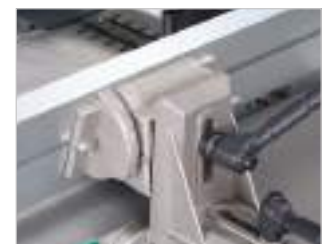
The aluminium jointing stop is pivoted continuously through 45°. The preset angle can conveniently be read off on a scale.
