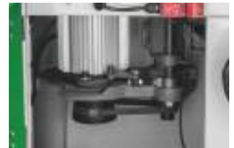
Fast and easy speed change thanks to multiple V belt
