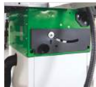
With two lateral extraction ports (Ø 100 mm)
