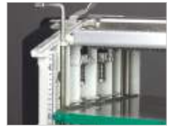
The spring mounted intake rollers prevent indentations on the wood. The thicknessing table is guided on four columns.
