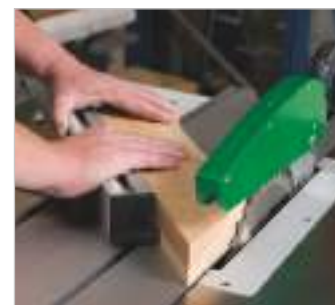
The cross cut stop supports mitre cuts on both sides, 45°
