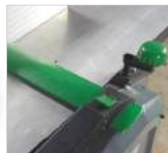
The planer knives are covered by a guard with a practical quick clamping mechanism. The desired chip removal can be set via a convenient hand crank for thickness planing of up to 2 mm. Easy to read off on the scale (fig. shows ADH 250).
