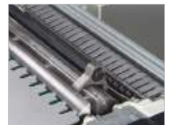
The planing knives are adjusted via the enclosed planing knife setting gauge.
