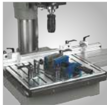
Machine vice can be clamped on table
