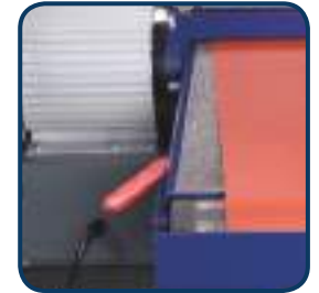
Graphite coating on the belt sanding machine improves the anti-frictional properties and the service life of the sanding belt
